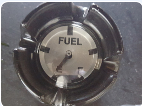
External Fuel Gauge allows for easy monitoring and filling.
